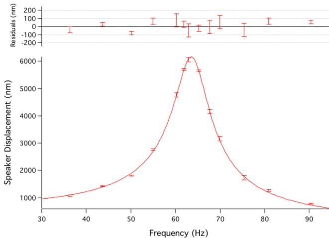
Fig. 3. Frequency response curve for the loudspeaker with corresponding residuals plot. The data were fitted to the equation for a driven, damped, harmonic oscillator.
